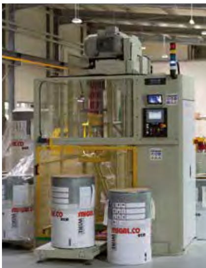
Respooler for twist-free drums
