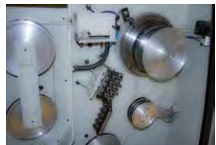
Twist-free drawing machine
